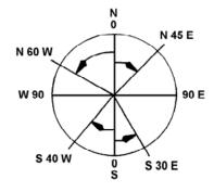
Figure 6. Bearings are read from a quadrant compass
