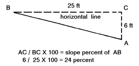
Figure 7. Method of determining slope percent.
