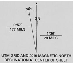
Adjusting values in a clockwise direction require addition of departure values. Adjustments in a counter-clockwise direction subtraction. For the Big Meadows VA quad MN is separated from GN by 9° 57' to convert to TN plus 1° 36' to convert TN to GN for a total positive difference of 11° 33', round off to 12°. Therefore,  $320^\circ + 12^\circ = 332^\circ$
