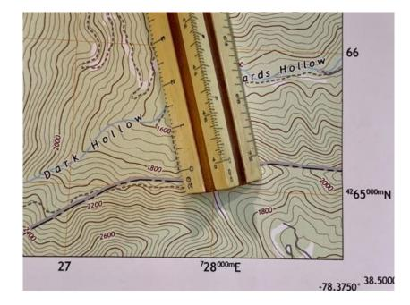
For the trail section in UTM 2765 located between index contour lines 1800 and 1600. The difference in elevation is 200-ft and the distance between the index contours is  $900^+$ -ft. Since the map scale is in 200-foot increments use 1000-feet for the distance. % slope = (200 | 1000) \* 100 = 20%
