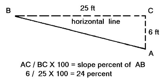
Figure 7. Method of determining slope percent.
